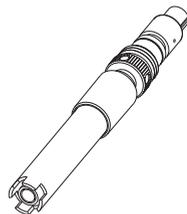
**HI 7609829-11:** The Chloride ISE is a combination solid state sensor used for the detection of free chloride ions in freshwater samples. The sensor utilizes a silver chloride pellet housed in a PEI head and a silver/silver chloride double junction gel filled reference electrode. This sensor is used in place of the pH sensor in the probe.
