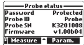
**Note** The probe status screen will automatically be displayed when the probe sensor status has changed. If this occurs, the "Measurement Screen" and "Parameter Selection" softkeys are available (see Section 5.2).
