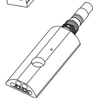
**HI 7609829-10:** Ammonium selective electrode (ISE) is a combination liquid membrane sensor used for the detection of free ammonium-nitrogen in freshwater samples. The sensor utilizes a polymeric membrane made with ammonium ionophore in a PVC head and silver/silver chloride double junction gel filled reference electrode. This sensor is used in place of the pH sensor in the probe.
