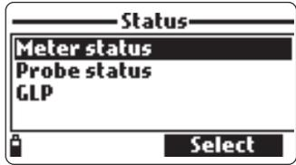
**Note** GLP data is stored for the last 5 calibrations. This calibration history allows the user to detect when readings start to change and sensors may require cleaning or replacement.
