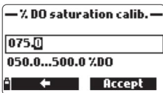
**Note** If the D.O. input is not within the acceptable range, the message “Invalid input” is displayed.
