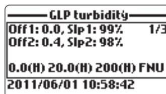
**Notes** If no turbidity calibration has been performed or if calibration was cleared using the "Restore factory calib." option the offset and slope values are set to default, and the message "Factory calibration" is displayed. Press <ESC> to return to the previous screen.
