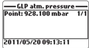
**Notes** If no atmospheric pressure calibration has been performed or if calibration was cleared using the "Restore factory calib." option the offset value is set to default, and the message "Factory calibration" is displayed. Press <ESC> to return to the previous screen.
