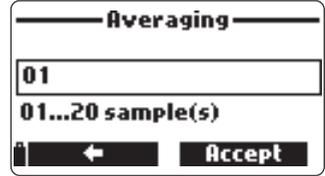
**Note** Each reading takes 1 second, so when logging the first sample will be delayed by a few seconds if averaging is used.
