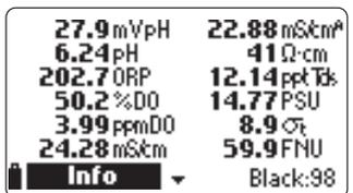
**Note** Details are available only for the enabled parameters.
