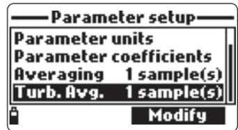
As is the case for the other measurements, averaging is useful to provide representative readings of the “average” value in flowing water. Turbidity averaging can be set separately because the optical turbidity sensor is more strongly affected by bubbles and debris in the water stream than the other sensors.
