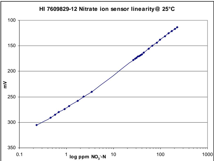
The calibration solutions and displayed measurements are as ppm Nitrate-nitrogen. Due to the space restriction of the display the unit of measurement will be displayed as “ppmNi”.
