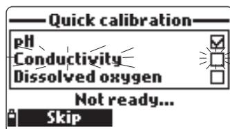
**Note** To bypass any of the calibrations press <Skip> to move to the next sensor in the quick calibration menu.
