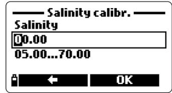
**Notes** These procedures calibrate the slope value. To calibrate the offset, set the calibration point at 0  $\mu\text{S}/\text{cm}$  and repeat the procedure.
