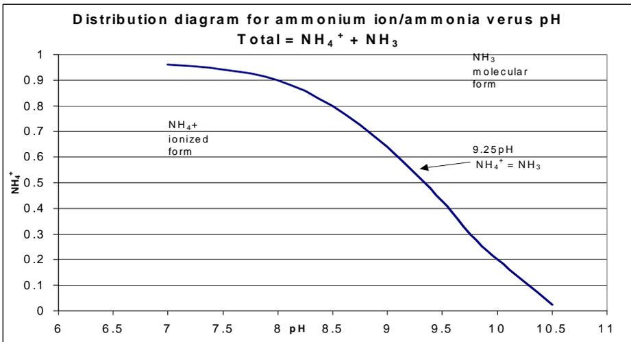
The HI 7609829-10 sensor is specified for 0.02 to 200 ppm (mg/L)  $\text{NH}_4^+$ -N (equivalent to 0.026-260 ppm (mg/L)  $\text{NH}_4^+$ ). Based on the corresponding molecular weights of nitrogen and ammonium, the relationship is:  $\text{NH}_4^+$ -N =  $(\text{NH}_4^+) \times 0.7778$ .  $\text{NH}_4^+$ -N is also called ionized ammonia. The sensor responds in a Nernstian manner (like a pH sensor) and produces a voltage that the meter converts to a concentration value.
