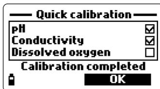
**Note** To quit the quick calibration procedure, press ESC at any time.
