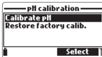
If a new pH sensor has been installed use "Restore factory calib." before performing a user calibration
