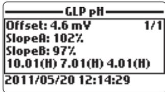
If a quick calibration was performed, the buffer values are replaced with the "Quick calibration" indication.
