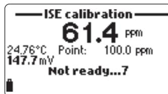
Position the sachet to ensure sensor membrane and ceramic junction are completely immersed in solution. A value close to 100 ppm and the message "Not ready..." will be displayed.
