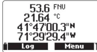
The GPS signal strength is always displayed through a 3 length antenna indicator on the bottom right corner of the LCD. If the antenna symbol is blinking, the satellite acquisition is not yet completed or the signal strength is not sufficient. Signal strength can be improved by moving outdoors and away from buildings and trees.
